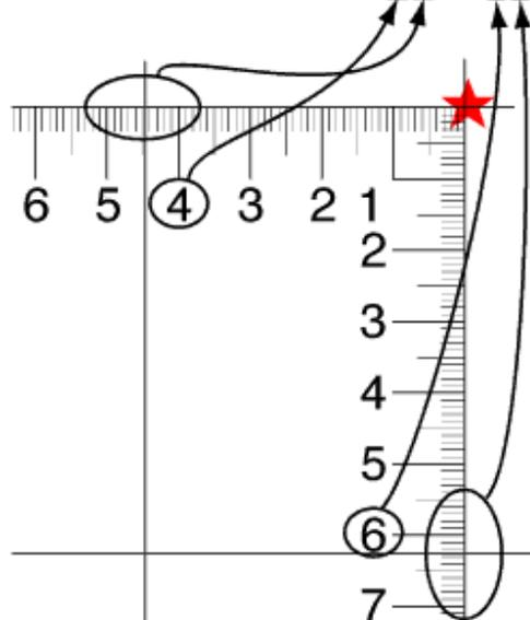
If you are using an odd scaled map or if you left your UTM tools behind, you can quickly make a simple corner ruler using the scale bars on the map.
